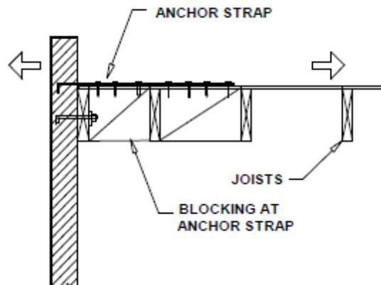
Figure 6-4 Wall anchorage
