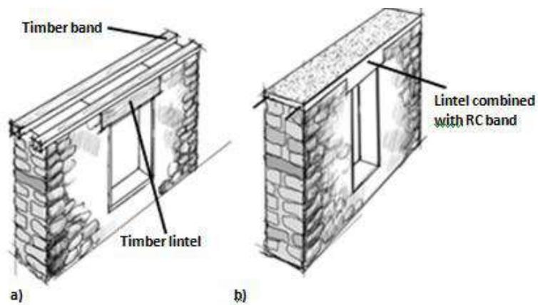
Figure 7-14 Combining floor/roof and lintel band: a) timber band, b) RC band
