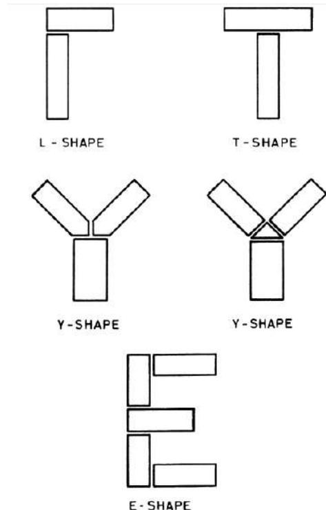
*Figure 4-4 Recommended shapes for buildings with irregular plans*
