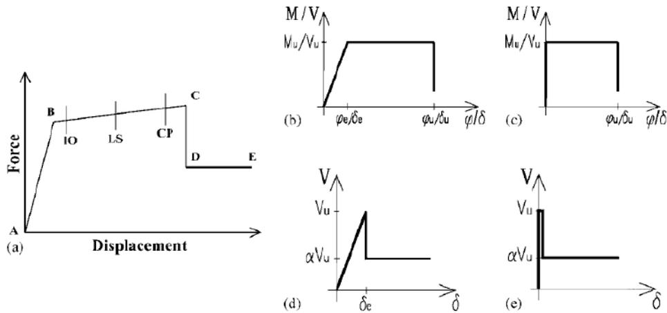
Figure 7-23 (a) Standard shape of the force vs displacement curve in SAP2000® v.10 for the plastic hinge element ; (b) and (c): behavior assumed, respectively, for the entire pier and the correspondent plastic hinge; (d) and (e): behavior assumed, respectively, for the entire spandrel beam and the correspondent plastic hinge.
