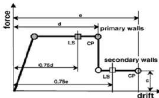
Figure 2.6 Generalized force deformation relation for masonry element and component (FEMA356)
