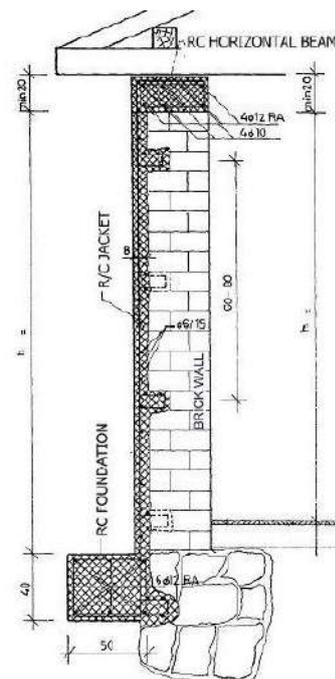
Figure 7-6 Application of RC coating
