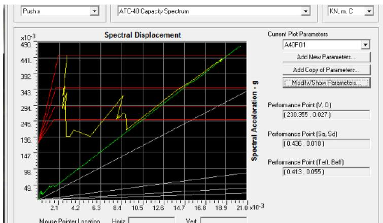
Figure 7-27 Push Over Curve of Local Building with lintel, rigid diaphragm and columns, from SAP 2000 v 14.0.0 Analysis
