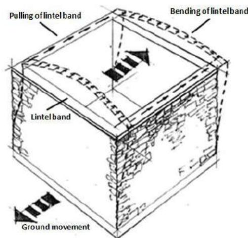
Figure 7-8 Pulling and bending of a lintel band in a stone masonry building (adapted from: Murty 2005)
