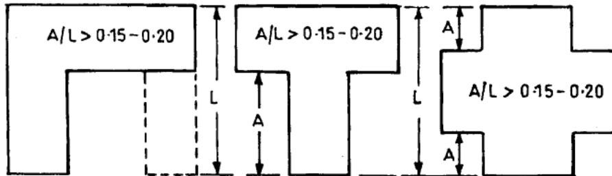
*Figure 4-3 Plan irregularity limits that require strengthening of overstressed elements and re-entrant corners*
