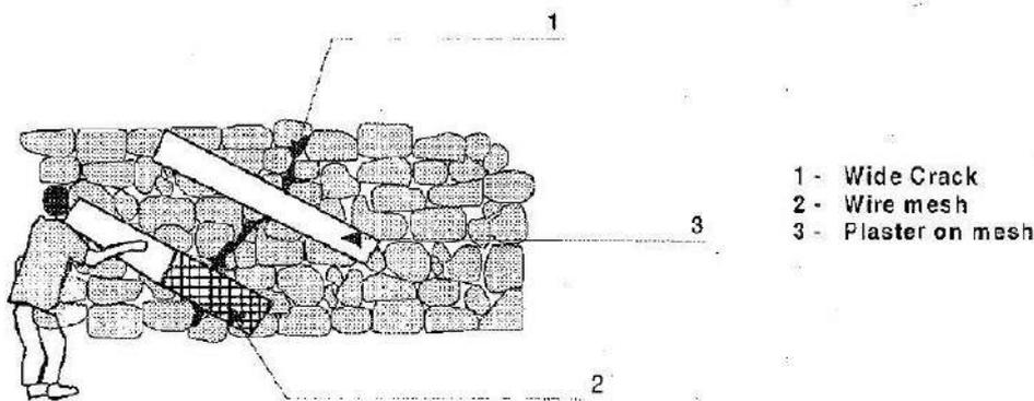
*Figure 7-5 Fixing mesh across wide cracks*
