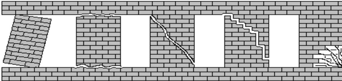
Figure 2-1 Different crack patterns of un-reinforced masonry pier
