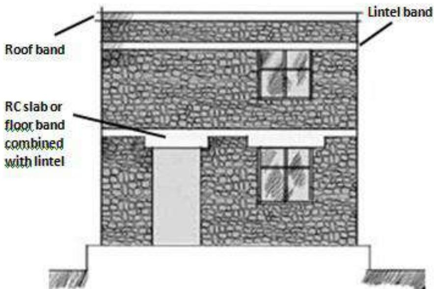
Figure 7-13 Merging RC floor and lintel bands
