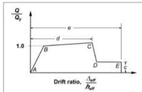
Figure 7-21 Generalized Force-Deformation Relationship for Deformation Controlled Masonry Elements or Components (FEMA 356-2000)
