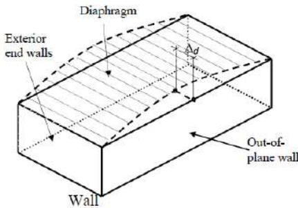
The behaviour of a flexible diaphragm under lateral load can be approximated as that of a wide flanged I beam with a large depth. The web of the I beam resists shear while the flange contributes to resisting moment generated by the uniform lateral load.
