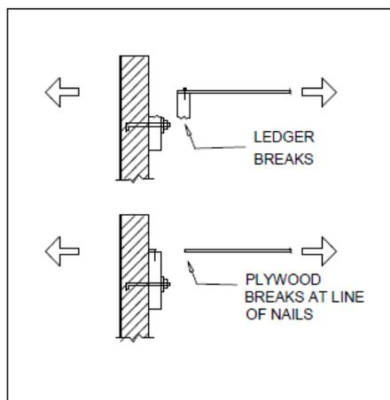
Figure 6-5 Connection relying in cross-grain of timber members induce cross-grain tension causing failure of the connection
