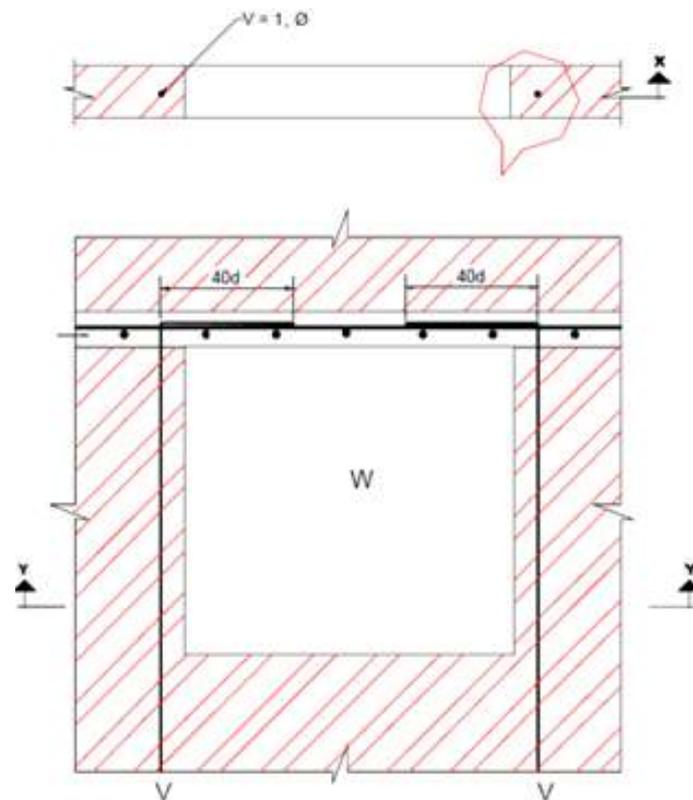
Figure 6-8 Reinforcement around opening in wall (Adapted from NBC 202)
