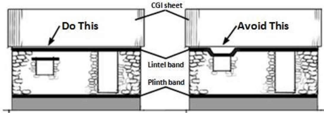
Figure 7-12 RC seismic bands should always remain level without any dips or changes in height (adapted from: GOM 1998)
