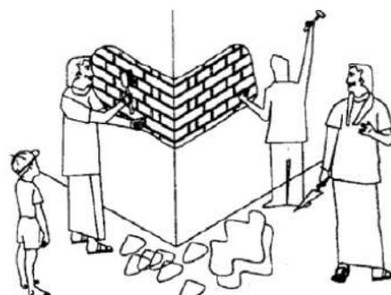
Fig.1:- Removal of Plaster & Raking of Joints
