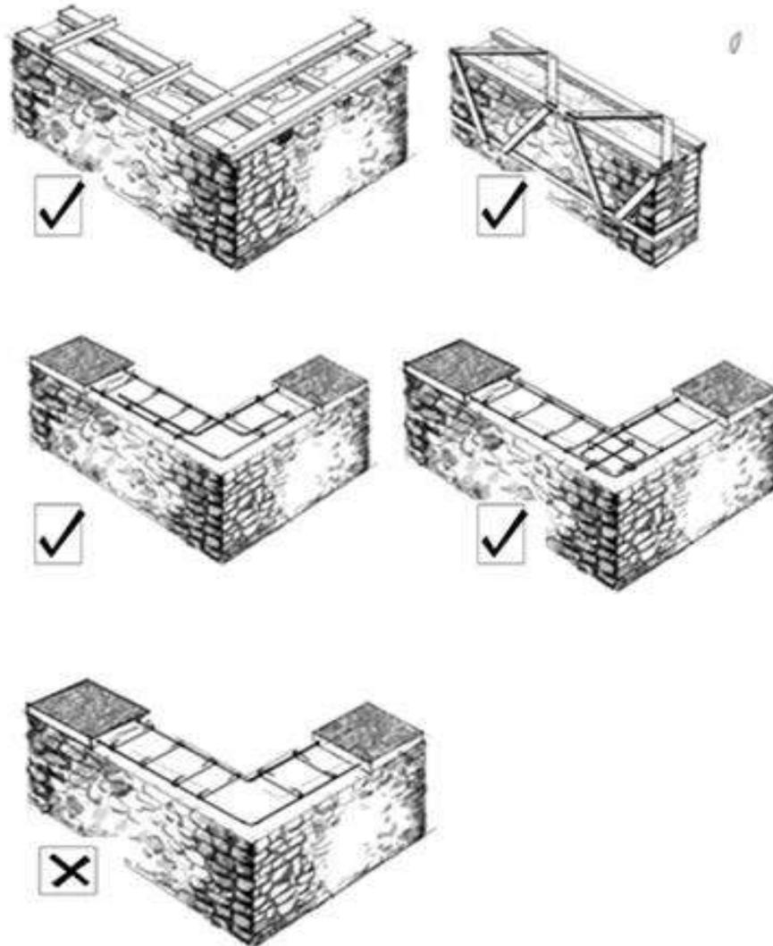
Figure 7-15 Recommended detailing of timber and RC bands (adapted from: T. Schacher and C.V.R Murty)
