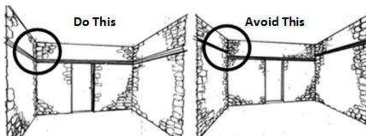
*Seismic bands must be continuous, like a loop or a belt.*
