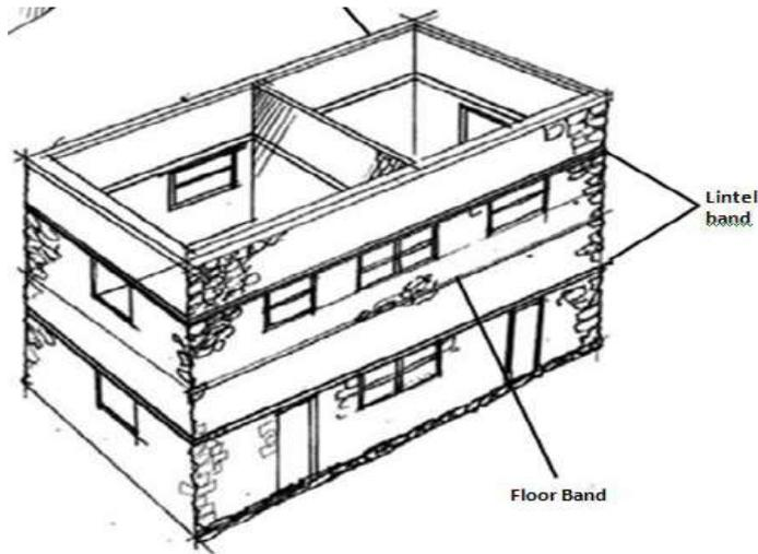
Figure 7-10 Location of seismic bands in a stone masonry building (roof omitted for clarity) (adapted from: UNCRD 2003)
