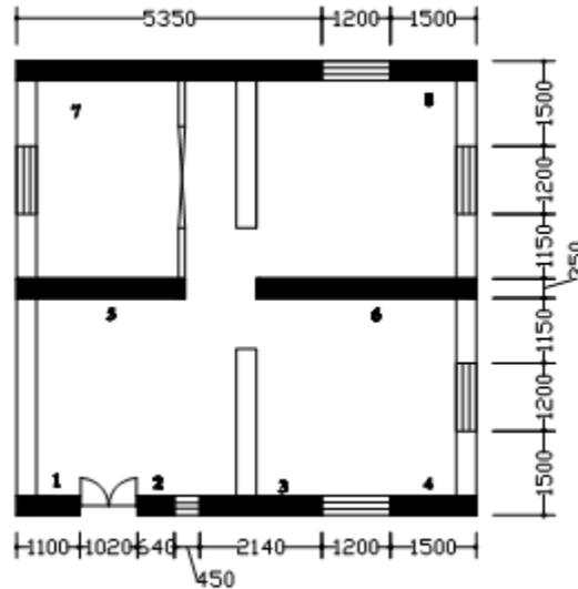
Figure 7-3 : A sample masonry building
