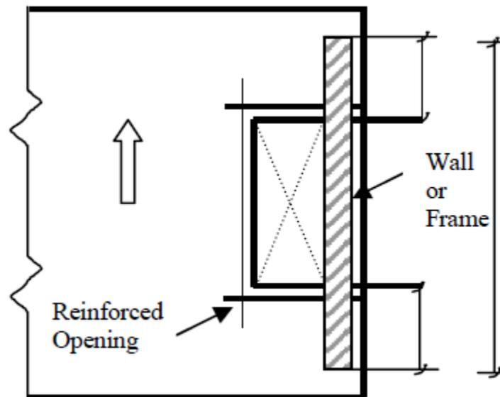
Figure 6-7 Opening adjacent to the masonry walls
