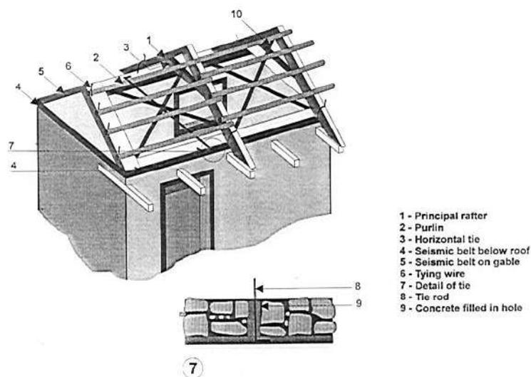
Figure 6-6 Stiffening of sloping roof structure
