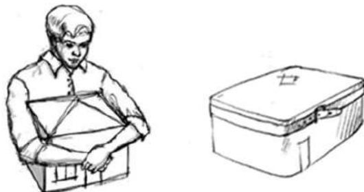
Figure 7-9 A seismic band acts like a belt (adapted from: GOM 1994)
