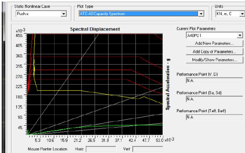
Figure 7-26 Push Over Curve of Local Building with lintel and rigid diaphragm, from SAP 2000 v 14.0.0 Analysis
