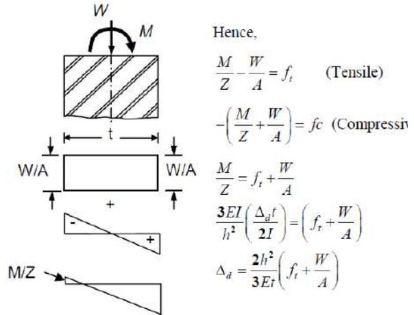
**Figure C36: Stresses at the base of wall**
