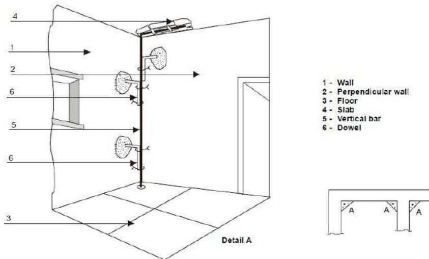
Figure 7-16 Vertical Reinforcement at corner and Junctions of Walls
