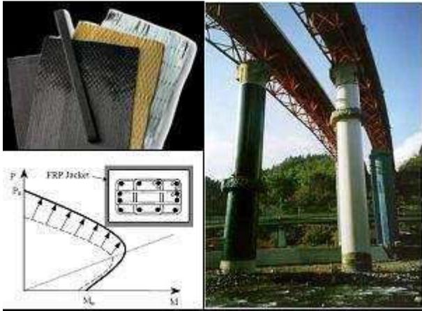
Figure 7-19 Different types and uses of Fibre wraps
