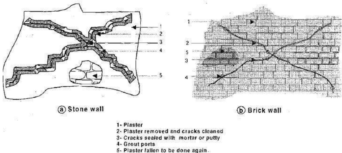
Figure 7-4 Filling grout in cracks
