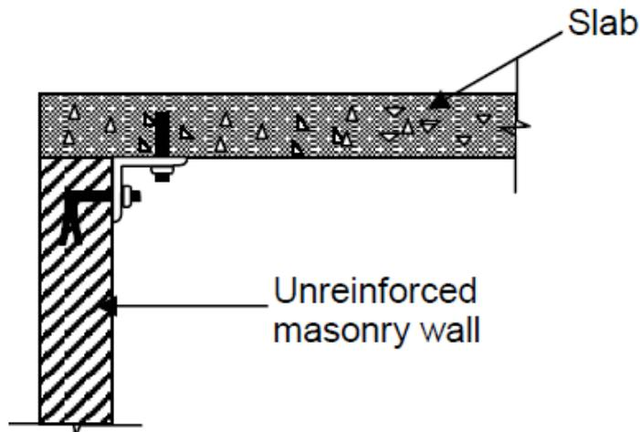
*Figure 6-3 Anchorage of RCC slab with masonry wall*
