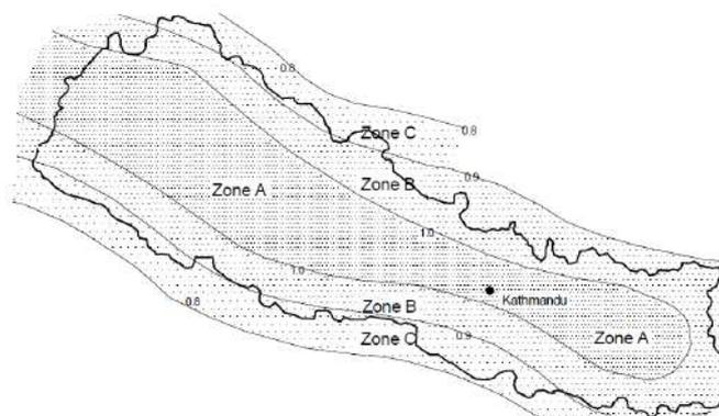
Figure 4-1 Seismic zones for masonry structures (NBC 109)
