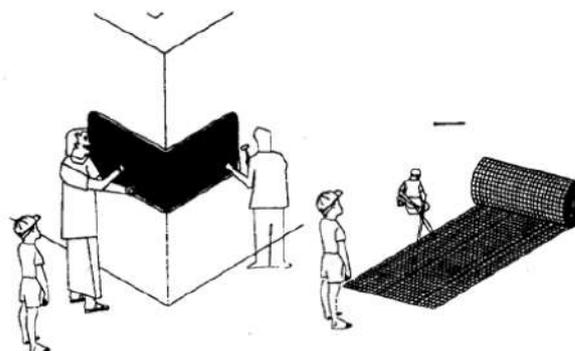
Fig. 2 :- Galvanised steel wire mesh
