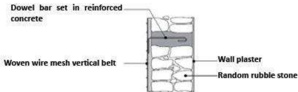
Figure 7-7 Single-sided jacketing showing steel dowels
