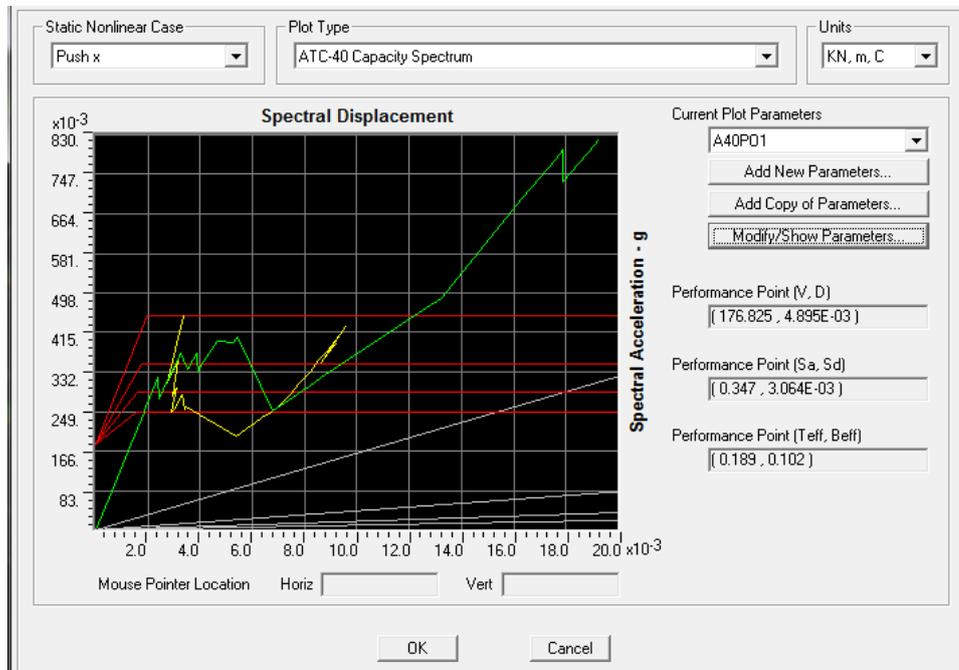
Figure 7-28 Push Over Curve of Local Building with lintel, rigid diaphragm and meshing, from SAP 2000 v 14.0.0 Analysis
